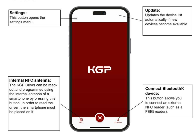
To program a driver, you can either use the internal NFC antenna of your phone, if available, or connect an external NFC reader via Bluetooth®.
